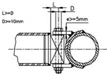
The removable connection type 3 (left) and type 4 (under) are only allowed for attaching roof reinforcement and optional members, and are forbidden for joining the upper parts of the main rollbar, the front rollbar and the lateral half-rollbars together.
