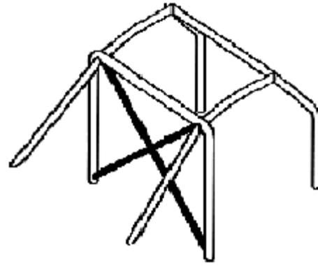
Diagonal member may also be designed as an inverted V, but then must also the roof reinforcement be shaped like a V.
