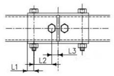
The removable connections type 1 (left) and 2 (left under & under) must be used for joining the upper parts of the main rollbar, the front rollbar and the lateral half-rollbars together.
