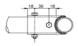
The removable connection type 3 (left) and type 4 (under) are only allowed for attaching roof reinforcement and optional members, and are forbidden for joining the upper parts of the main rollbar, the front rollbar and the lateral half-rollbars together.
