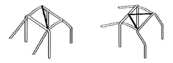
Tube which runs longitudinal from one of the highest points of the B-bar to the other side of the Abar, must also be reinforced in each corner according to the drawing beside. A space of minimum five cm between helmet and tubes is recommended.
