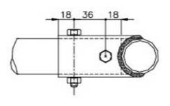
The removable connection type 3 (left) and type 4 (under) are only allowed for attaching roof reinforcement and optional members, and are forbidden for joining the upper parts of the main rollbar, the front rollbar and the lateral half-rollbars together.
