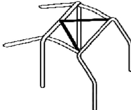
Tube which runs longitudinal from one of the highest points of the B-bar to the other side of the A-bar, must also be reinforced in each corner according to the drawing beside.
