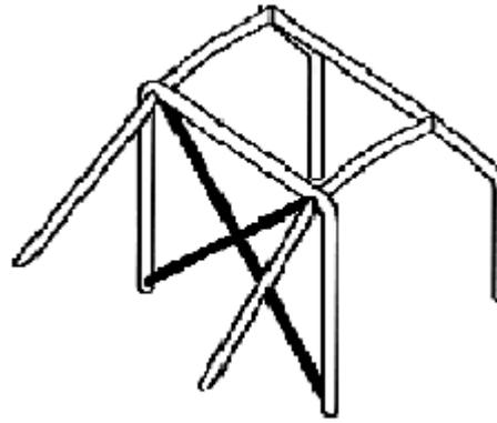
Diagonal member may also be designed as an inverted V, but then must also the roof reinforcement be shaped like a V.
