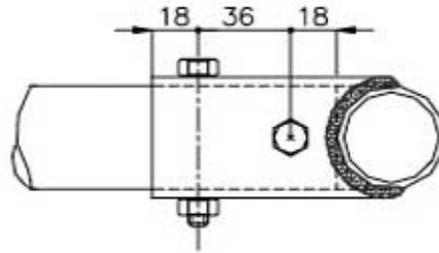
The removable connection type 3 (left) and type 4 (under) are only allowed for attaching roof reinforcement and optional members, and are forbidden for joining the upper parts of the main rollbar, the front rollbar and the lateral half-rollbars together.
